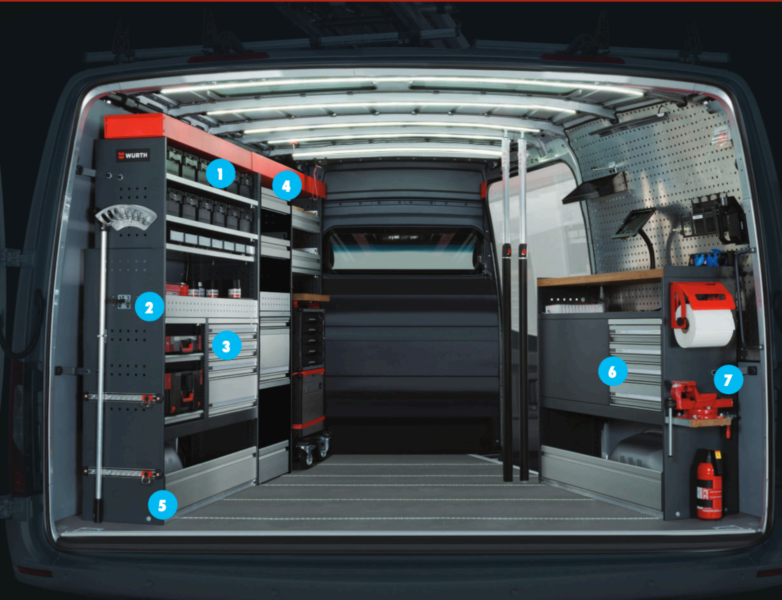
1 Storage bin shelves with patented front flap: for clear storage and easy access to small parts
